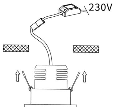
4. Adjust the luminaire. Shut on fuse in fuse box. The luminaire can be used now.
