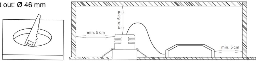
2. Shut off fuse in fuse box. Connect luminaire to driver only after power-off.
