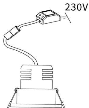
3. Connect driver to the mains supply and install luminaire in the ceiling according to below sketch.
